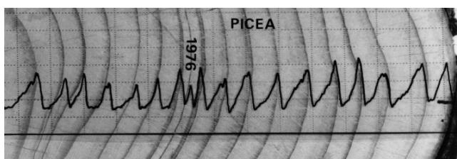
**Fig. 4: If the needle penetrates the tree rings of conifers nearly perpendicular, the profile reveals differences in density between earlywood and latewood; in this profile of a spruce tree, felled in 1986, the extremely dry summer of 1976 can be identified by the correspondingly narrow tree-ring with only a few latewood cells**
