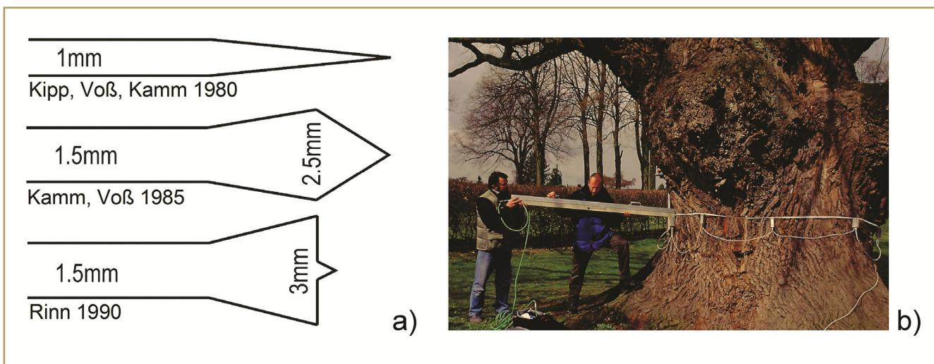
**Fig. 3: a)** A needle shaft of 1.5 mm and a flat tip of 3.0 mm width were found to be a good compromise for achieving maximum resolution and stability at lowest damage to the sample; **b)** With this needle, it was possible to drill up to a depth of 1.5 m into old oak trees and still detect tree-rings narrower than 0.5 mm (Rinn, 1990)
