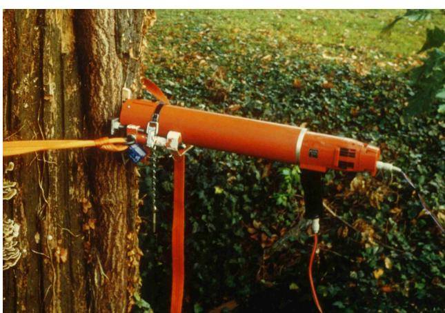
**Fig. 2: Resistance drill of the first portable device series from 1987, sold to experts worldwide; using such a machine, Ehlbeck and Görlacher proved a linear correlation of the profiles to wood gross density (1990)**
