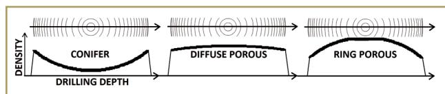
**Fig. 8:** Typical mean trends of drill resistance profile trends from radially drilled cross section (of calibrated machines without shaft friction), reflecting typical radial stem density trends as confirmed by x-ray measurements (Read et al., 2011)
