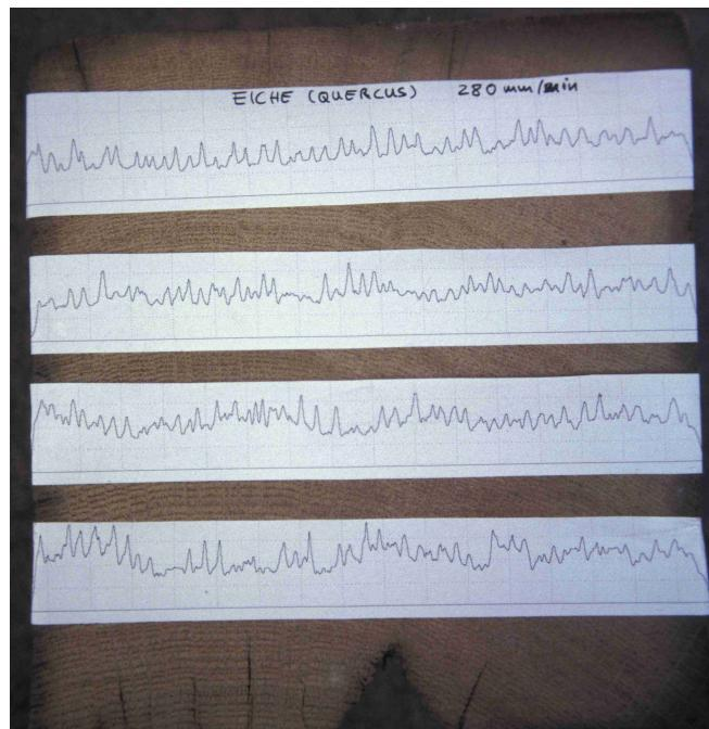
**Fig. 10:** Profiles of tangential drillings in oak often look like radial drillings in spruce and stay on one level due to the missing change in density in this direction; therefore, without knowing the species, drilling point and drilling direction, it is impossible to interpret the profiles correctly
