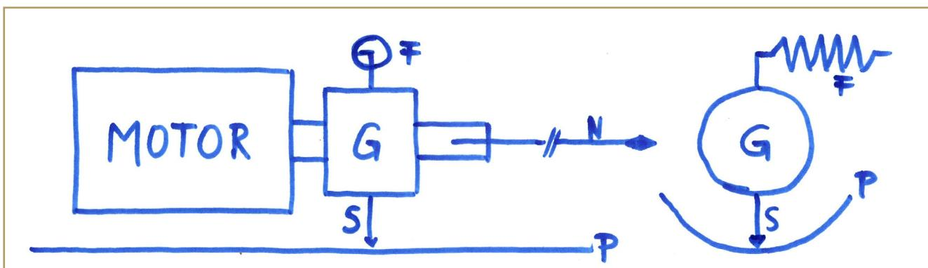
**Fig. 1: Sketch of an early resistance drill from 1984: a scratch pin (S) was fixed at a spring (F) loaded gear box (G) between motor and needle (N), creating a 1:1-scaled resistance profile on a wax-paper strip (P); because resonance and threshold effects due to the spring-loaded recording mechanism delivered systematically wrong profiles that were easily misinterpreted, this approach was abandoned and replaced by electric recording of motor power consumption**
