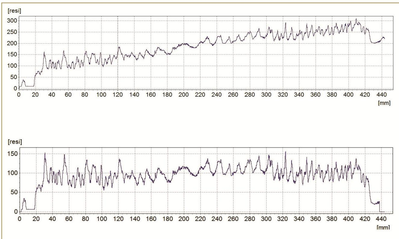
**Fig. 11: Depending on machine and needle type, shaft friction may lead to a more or less strong increase of the profile as the needle penetrates the wood (top profile); this effect can mask profile decline by decay and make interpretation more difficult; in case of doubt, reference drillings are required; the profile can be de-trended with a software, shown in the lower profile or a calibrated machine has to be used**
