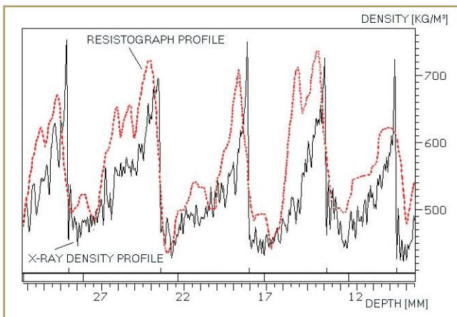
**Fig. 5:** This superposition of a radial x-ray density profile (resolution 1/100 mm) of larch with a resistance drilling profile shows that local wood density is the main factor determining drill resistance; the slope of the resistance profile at the tree-ring border represents the step function response of the method and thus represents the resolution limit of tree-ring detectability when penetrated perpendicular
